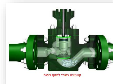
NPSH Net Positive Suction Head
